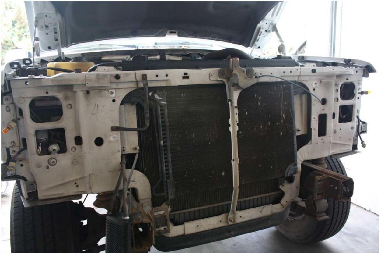
Step 2 - Mark the front support bracket even with bottom of hood latch assembly.
