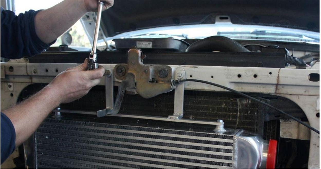
Step 10 – Install lower cooler mounts and drill mounting holes in the radiator support. Be sure to protect the radiator from puncturing using small piece of plywood or metal as shown in picture.
