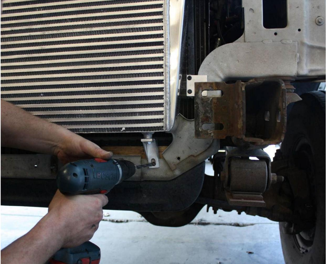
Step 11 – Install the original power steering cooler using supplied aluminum bracket. You will need to drill two mounting holes in the frame rails to secure the bracket as shown in the photo.
