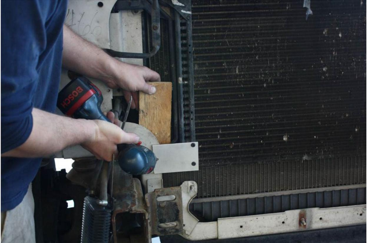
Step 6 - Cut off studs located below ac condenser mounts for intercooler clearance.
