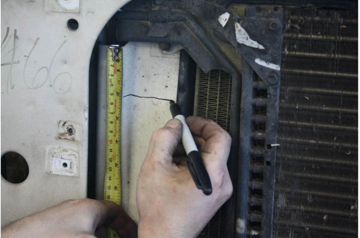
Step 8 - Next remove both left and right radiator side support brackets and cut along marked line as shown in picture. Then re install both brackets in their original location.
