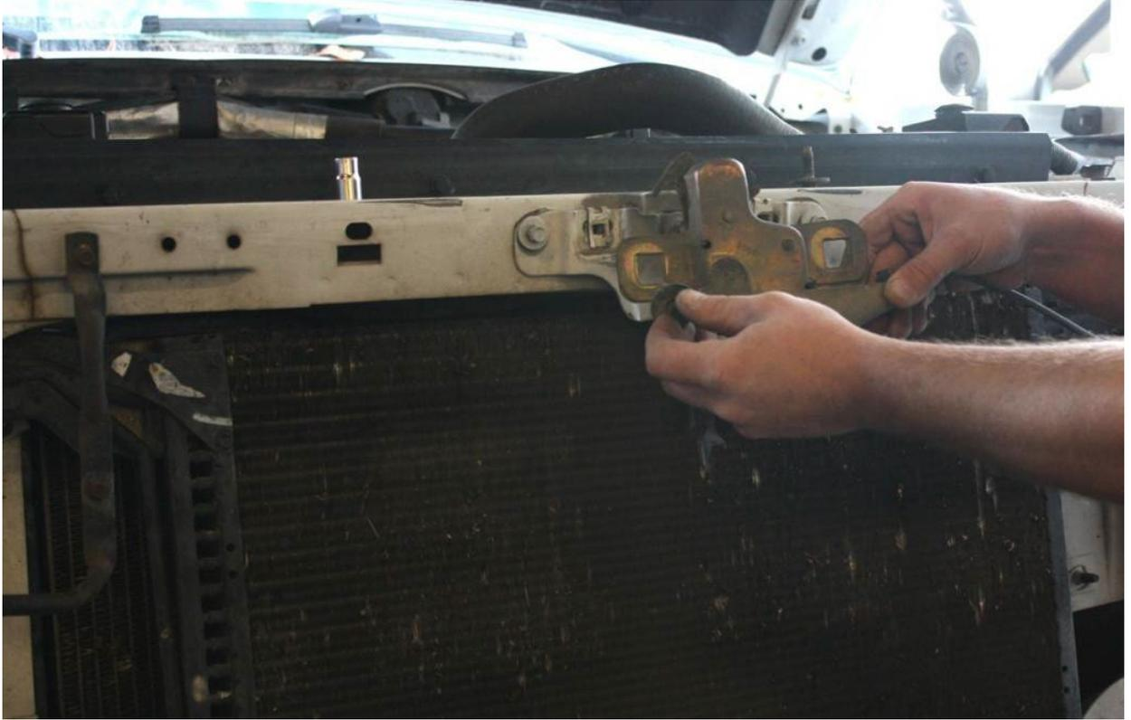
Step 4 - Remove both lower AC condenser brackets.
