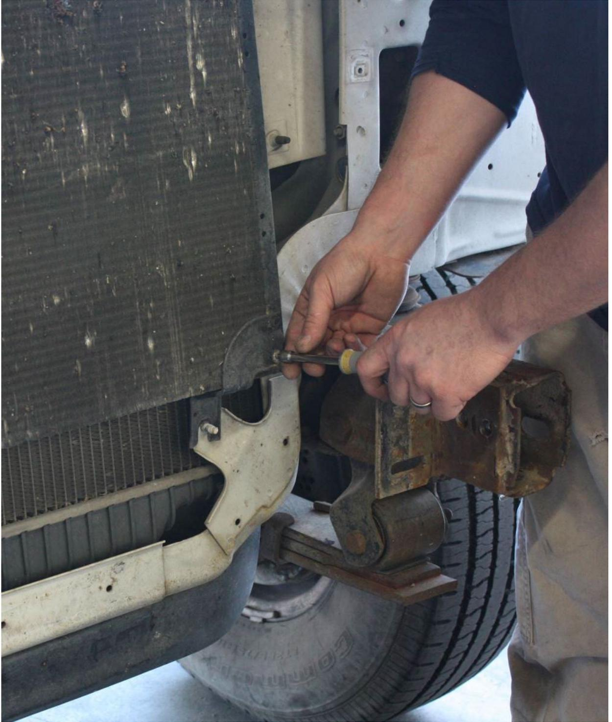
Step 5 - Install supplied new aluminum brackets. You will need to drill a mounting hole for each bracket. Use a small piece of plywood or metal to protect radiator from being damaged by the drill bit during this process.
