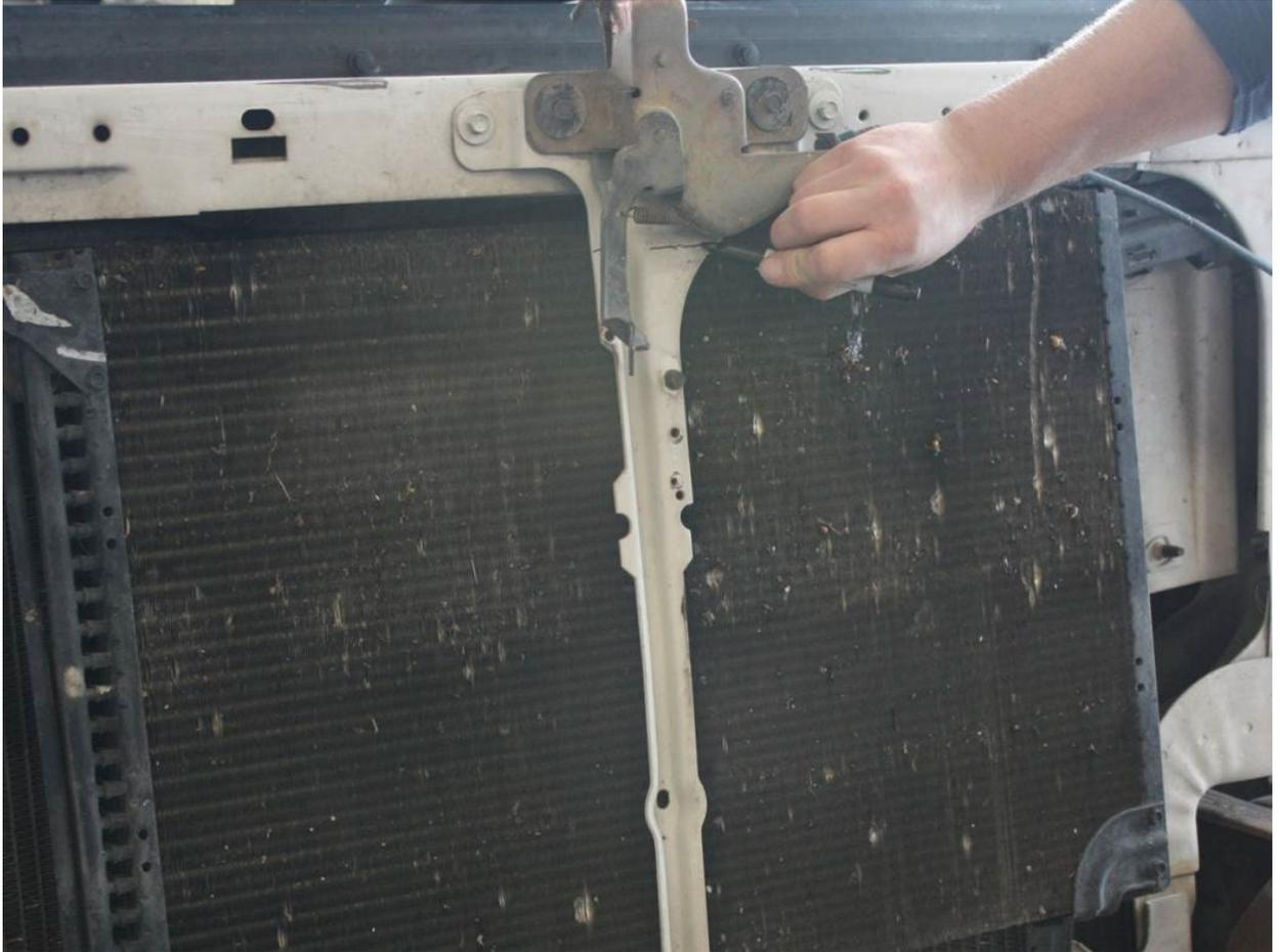
Step 3 - Discard lower portion of the support. Re install hood latch assembly along with trimmed support.
