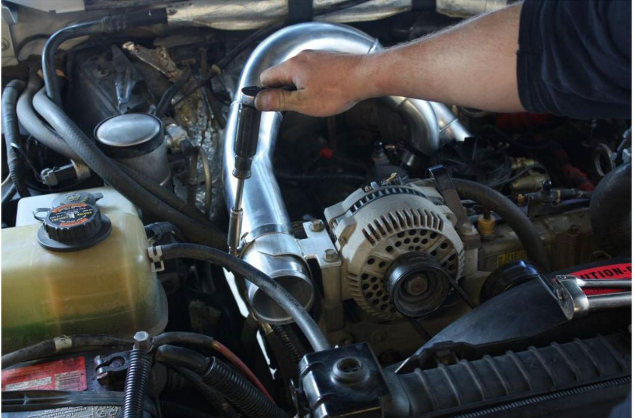
Step 15 – Install the new turbo pressure discharge tube using supplied mounting bracket and V-band clamp.
